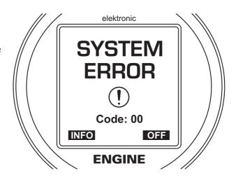
**A** Do not try to repair the instrument yourself. Contact a distributor or the producer with the 2-digit number specifying the error.
