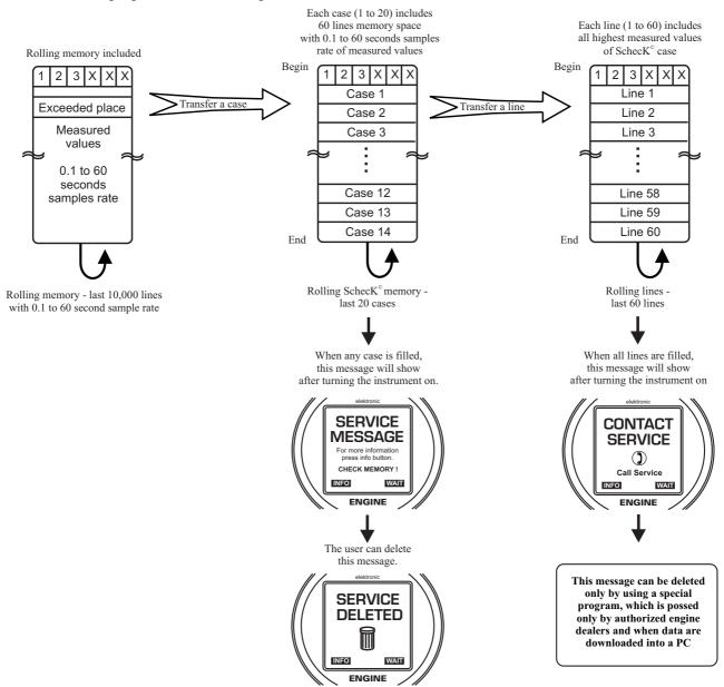
Cases 1 to 20 include the record of limit-exceeding values and engine hours, date and time referring to the moment of limit exceeding. Each case includes 60 lines.
