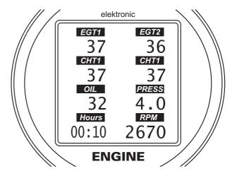
**A** If the instrument has not been purchased as a part of the engine, the configuration is required. Do the configuration with use of the Windows program delivered with the instrument.
