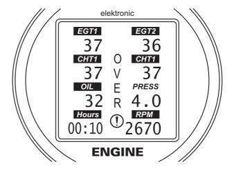
The limit value check is activated immediately after the set rotation value for the activation is reached. Only the minimum oil pressure check is activated after 5 seconds to allow the oil circuit to get pressurized.
